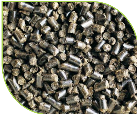
Wood pellets made of compressed saw dust – an example for organic renewable fuel
